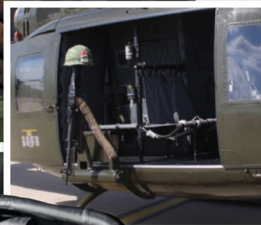
Below: Huey gunships were usually fitted with a machine gun operated by a door gunner along with other adaptable weapons such as rocket pods
